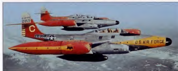
Below: Although possessing a good endurance and potent weapons load, the sluggish Scorpion was disliked by day-fighter pilots. The F-89Ds pictured carry underwing tanks for increased range.
